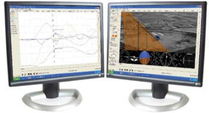
3-D playback of the flight ribbon provides a reference for ground track and altitude changes. 2-D graphs depict the relationship between flight variables such as speed and altitude.
