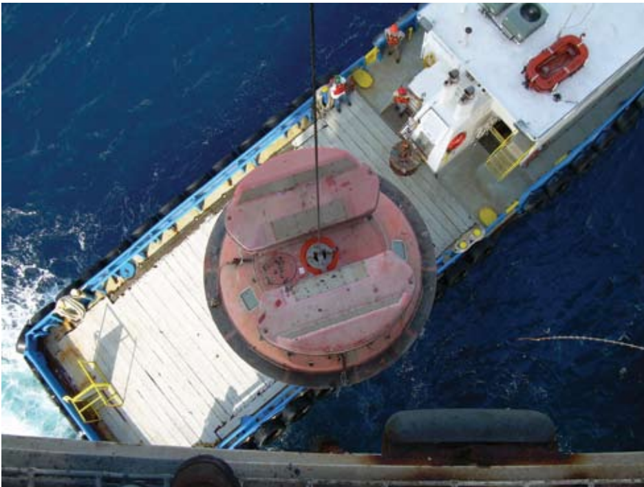
A Merit Energy escape capsule is loaded onto a work boat for repair.
