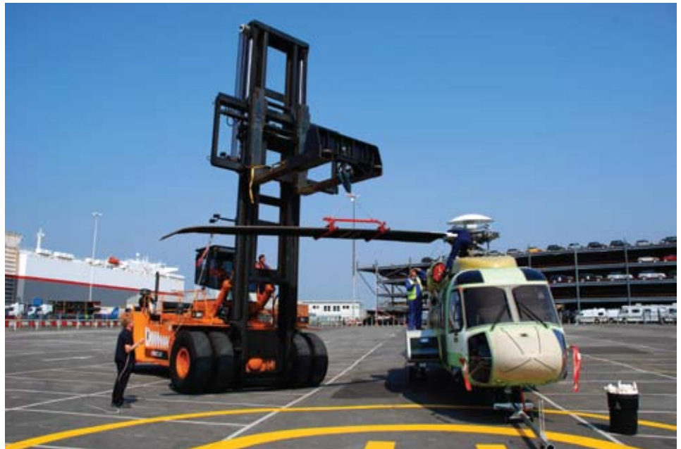
Blades are refitted in Southampton.
